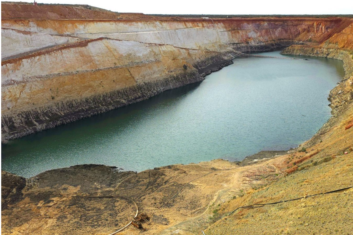
Figure 3 – Youanmi Main pit approximately 50% dewatered
