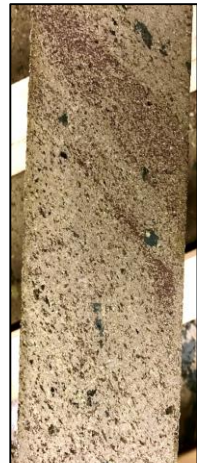
Sphalerite and pyrrhotite in SBJK170003
