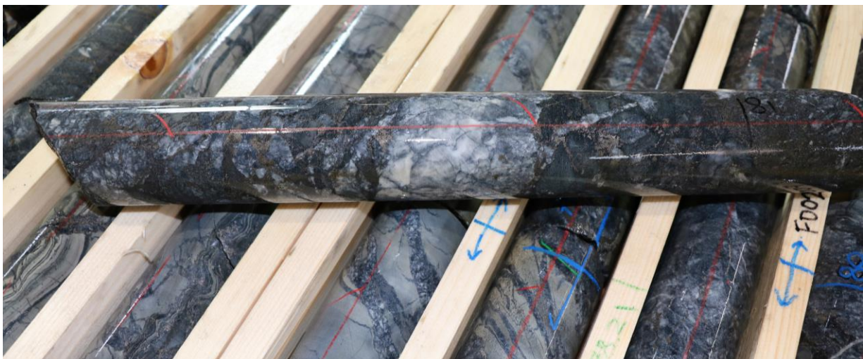
Figure 9. Quartz-carbonate-sulphide veined breccia, with quartz-carbonate-sulphide veined albitites in background from FAKD0006.
