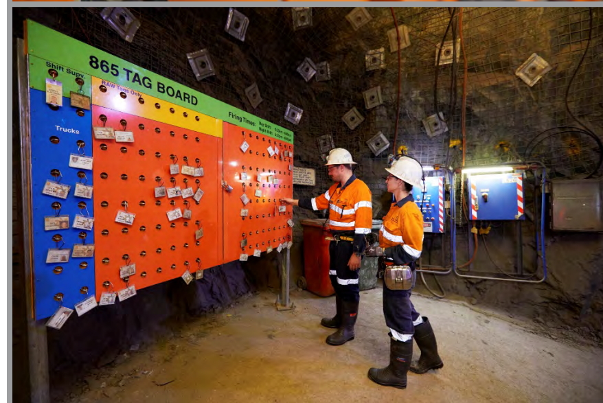
Above – isolation tag in an MCC room at Gwalia, WA. Below – the 'tag board' at 865 metres below surface, Gwalia, WA.
