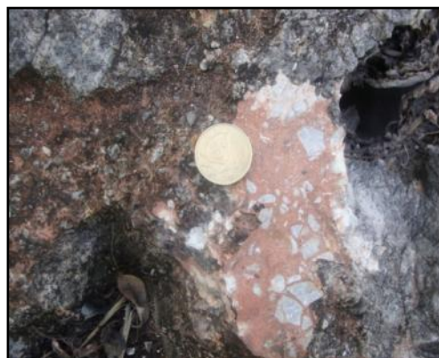
Figure 8 – Hematitic breccia containing disseminated copper lead and zinc minerals, at Lucas Post.
