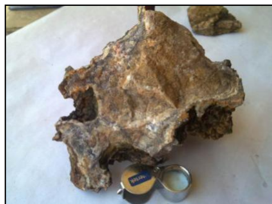
Figure 7 – Strongly mineralised rock from Lucas Post, showing pervasive oxidation. Darker patches are rich in copper, lead and zinc, whilst brown zones are highly anomalous in the base metals.
