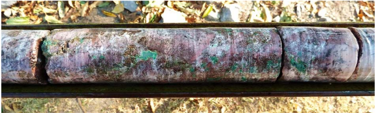
Drill core from GCDD0002 – copper mineralisation visible as green malachite, with chalcocite and minor chalcopyrite.
