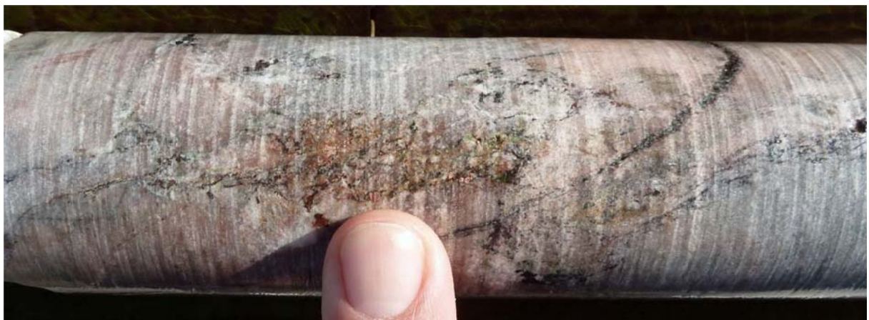
Drill core from GCDD0002 – visible 'native' copper mineralisation.
