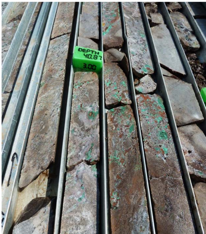
Drill core from GCDD 001 – copper breccia mineralisation clearly visible as green malachite & brown-grey zones containing chalcocite
