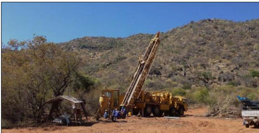
Figure 5 – RC drilling at Schlangental (Guchab Mountain in the background).
