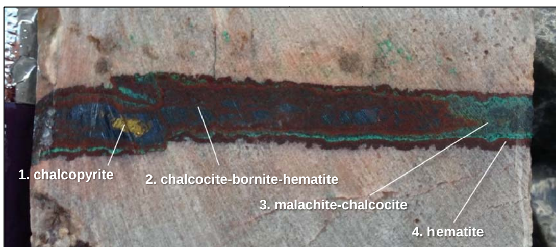
Figure 1 – A 5mm thick zoned copper-rich vein from GCDD0023 at Guchab. The vein originally would have been uniform chalcopyrite, with the zonation depicted entirely due to weathering. From freshest (1 – chalcopyrite) through to most weathered (4 – hematite), this zonation is indicative of the weathering processes at the Guchab Canyon deposit. Most of the deposit drilled to date is in weathering zone 3, comprising a malachite-chalcocite assemblage.
