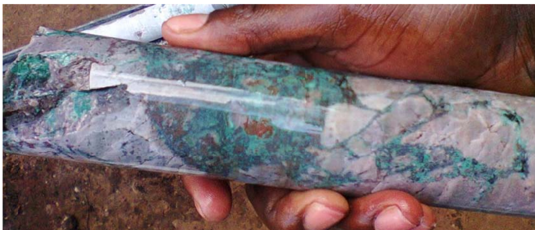
Breccia-hosted copper carbonate & sulphide mineralisation from GCDD0025 at Guchab.
