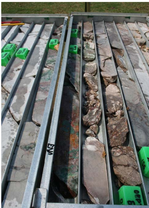
Figure 10 – Diamond drill core from Pad Two (GCDD0006) showing strong copper mineralisation.
