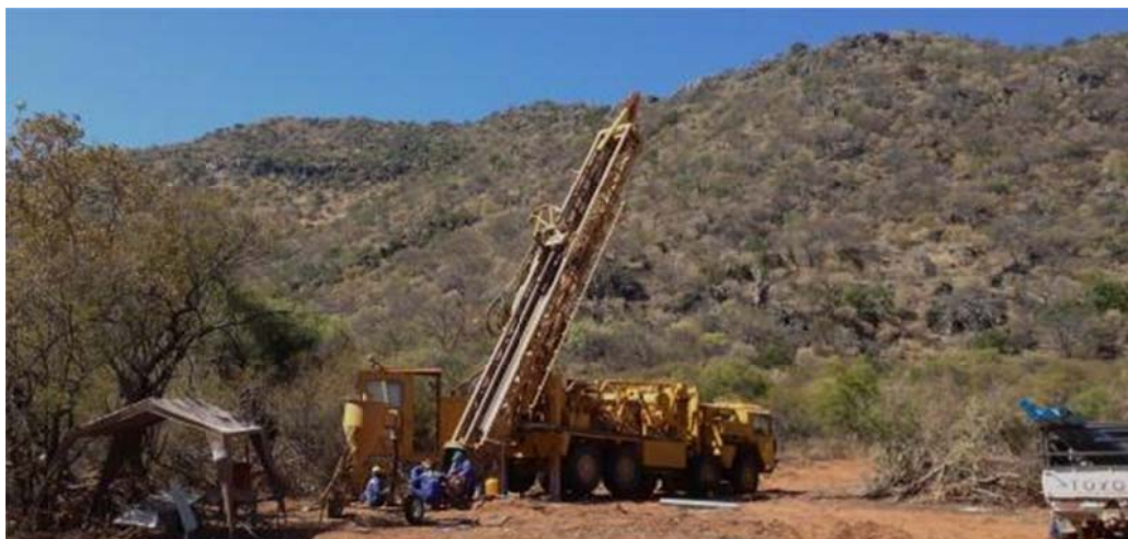
Figure 11 – RC drilling in progress at Schlangental.
