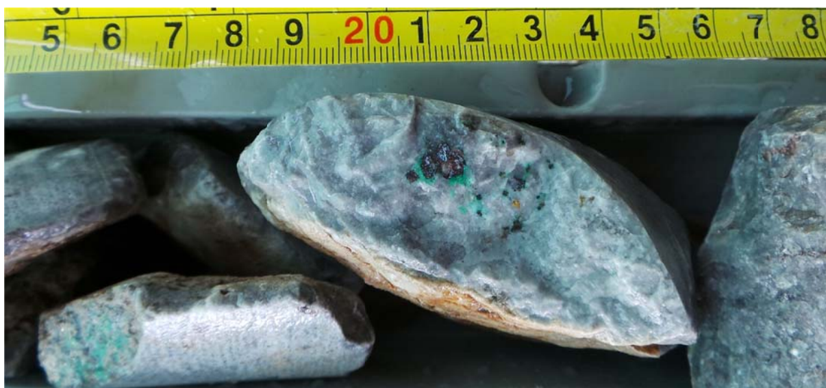
Figure 6 - Chalcocite (black-grey) and malachite (green) mineralisation in silicified dolomite at Guchab South, GCGDD0006 1.65m
