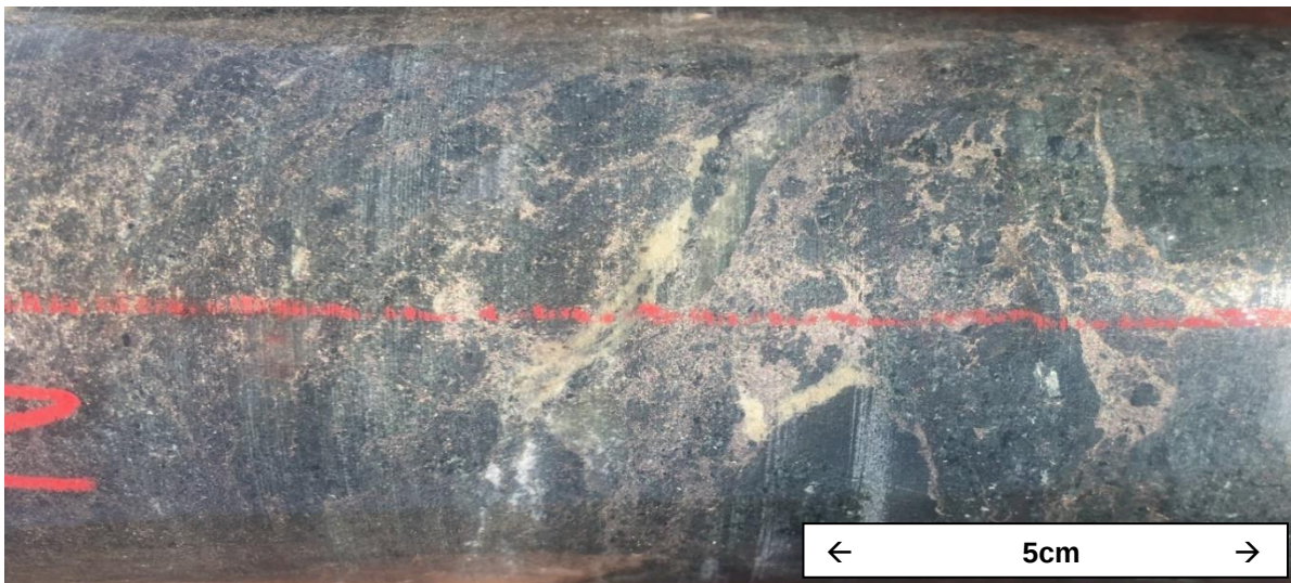
Photo 1: SBDD002, 425m. Massive/matrix sulphide breccia with pyrrhotite, pentlandite and chalcopyrite
