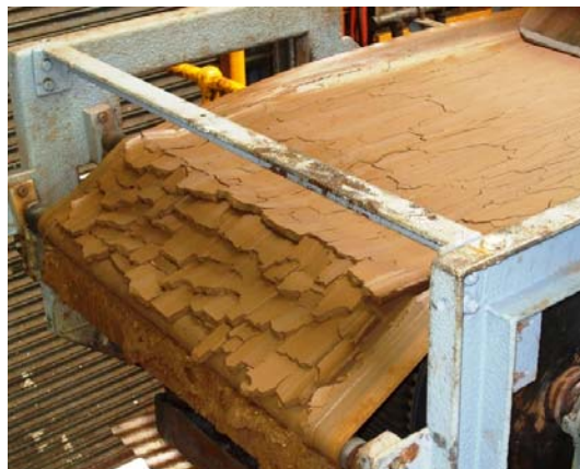
The high-zinc, low-iron non-magnetic fraction of EAF dust after magnetic separation
