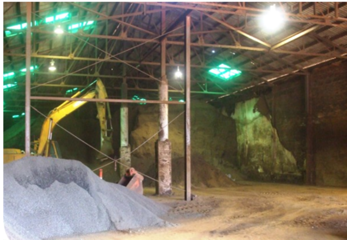
Operations at the Victorian zinc oxide production site. Crushed Zeehan feedstock may be seen in the left foreground, with EAF dust stockpile excavation at rear.
