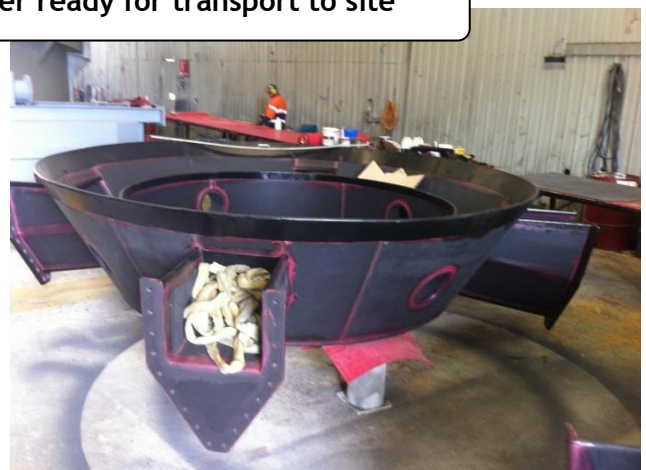
Float Cell and Float Cell Launder ready for transport to site
