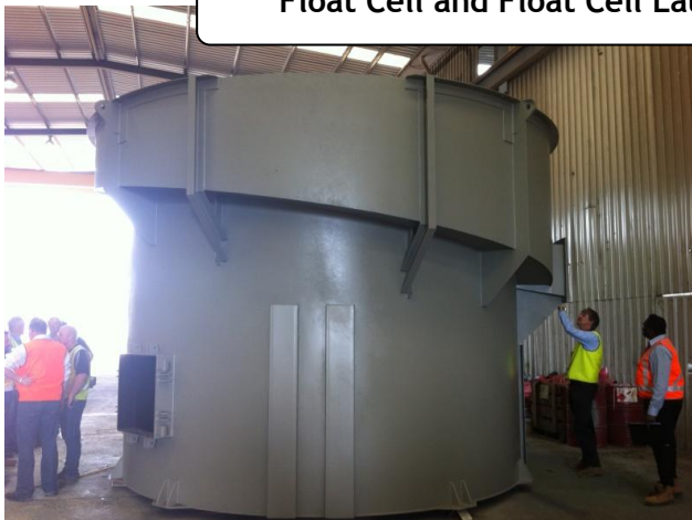
Float Cell and Float Cell Launder ready for transport to site
