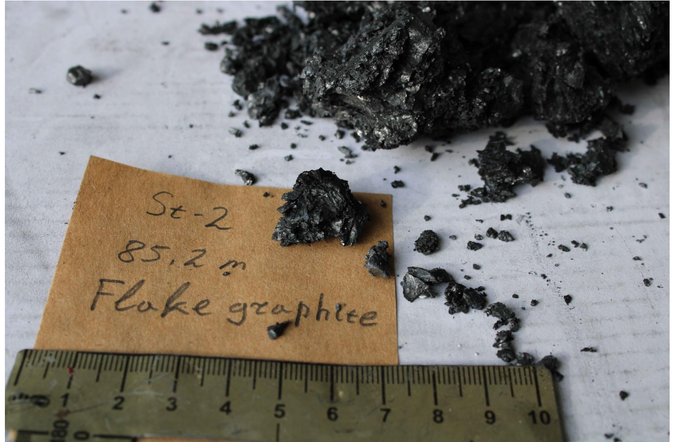
Flake graphite from the Sarytogan Graphite Deposit
