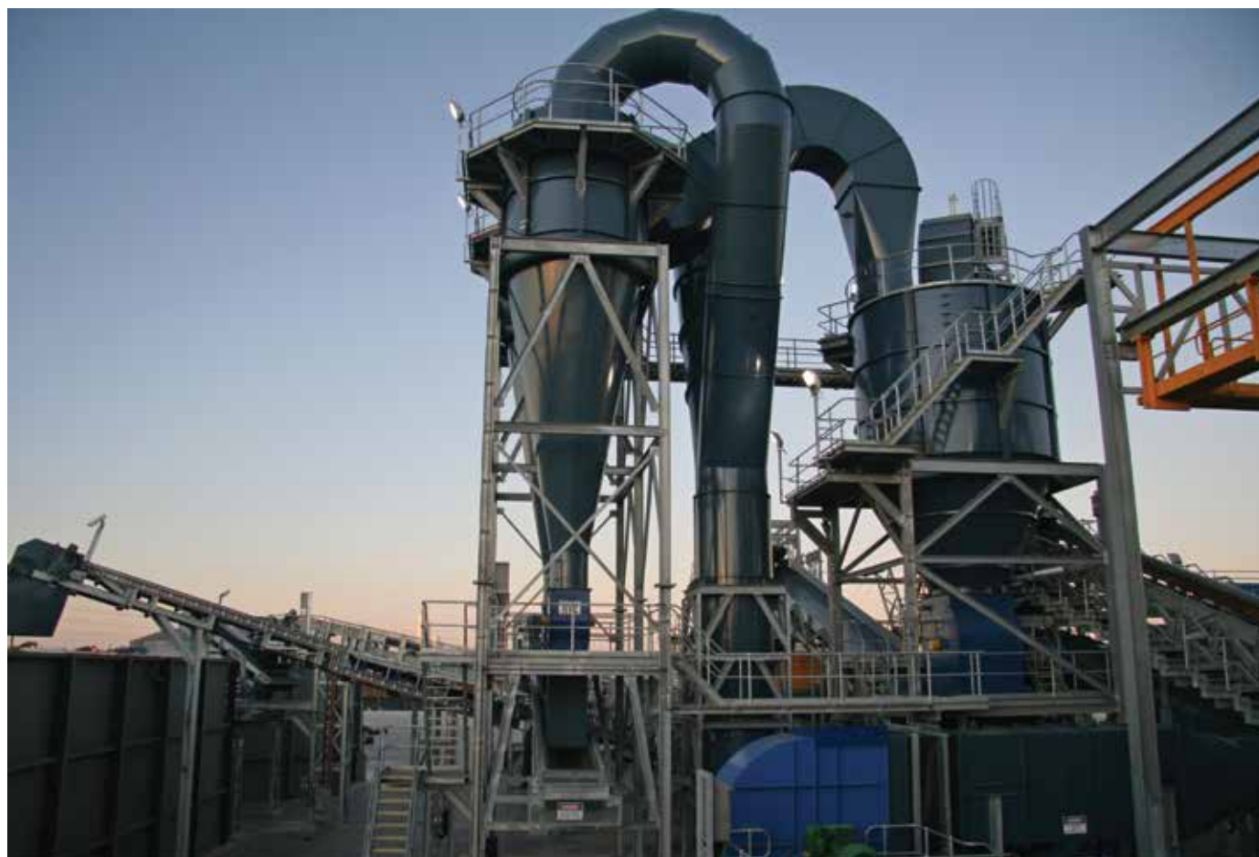
Kwinana, Western Australia: Newly installed mid-sized metal shredder (expansion box, cyclone and draft fan featured in the centre of the photo).
