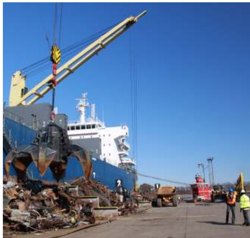
Loading heavy melt scrap into a bulk carrier for deep-sea export in Providence, Rhode Island
