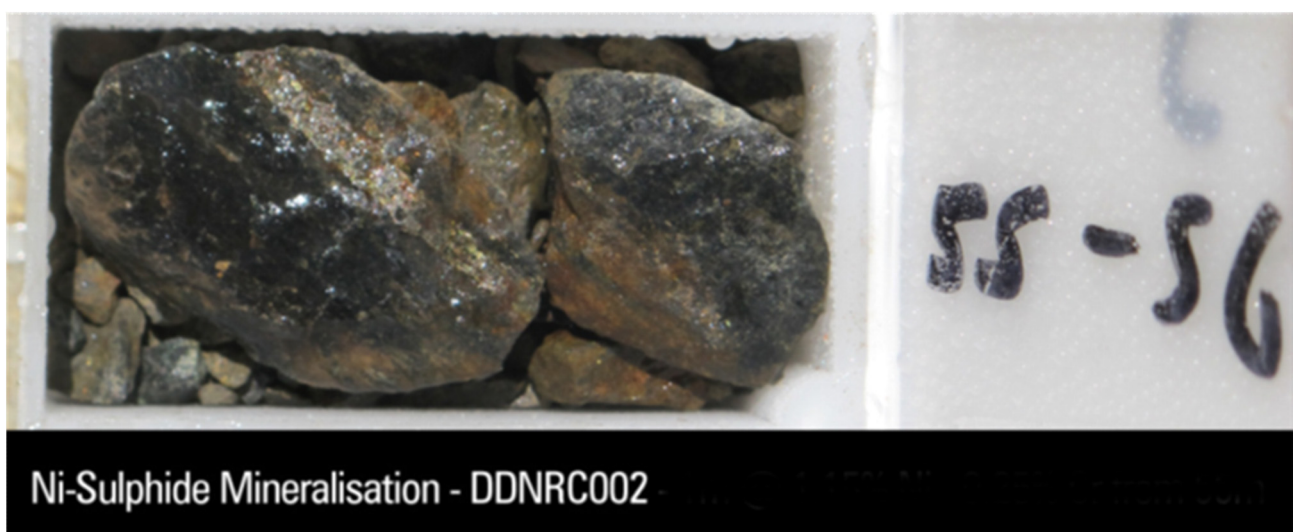
Figure 2 – Visible massive nickel sulphide stringers intersected in DDNRC002 between 55m – 56m down hole. The sulphides lie within a fresh rock intersection of 2m @ 1.08% Ni from 55m.
