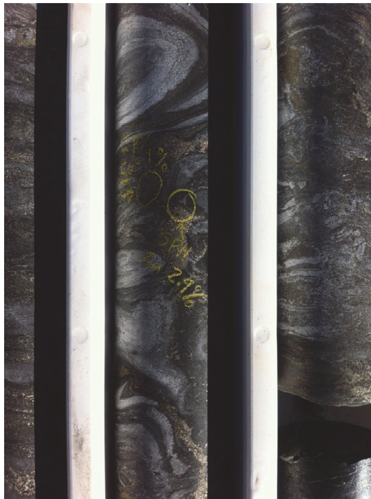
Figure 2 – a photo of drill core from DDRDD0005 at approx. 296m downhole. Chalcopyrite and sphalerite are visible in this sulphide rich interval. XRF analysis returned spot values of 2% Cu and 2.9% Zn. The widespread base metal mineralisation encountered by drilling supports the growing potential for major VMS-style mineralisation at East Laverton.
