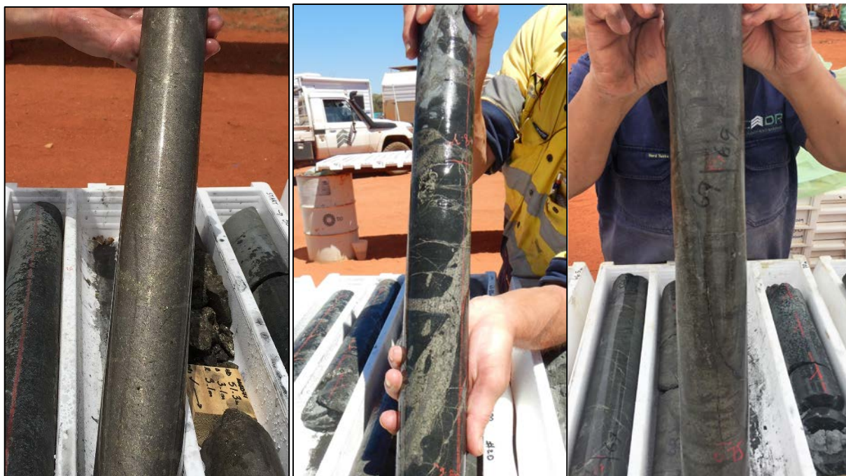
Figure 1 – Above left : drill core from the 17.45m high-grade intersection in MAD71. The section of drill core is from the massive sulphide interval that returned assays of 2.02m @ 5.05% Ni, 2.01% Cu, 0.21% Co and 3.31g/t total PGEs from 50.6m.
