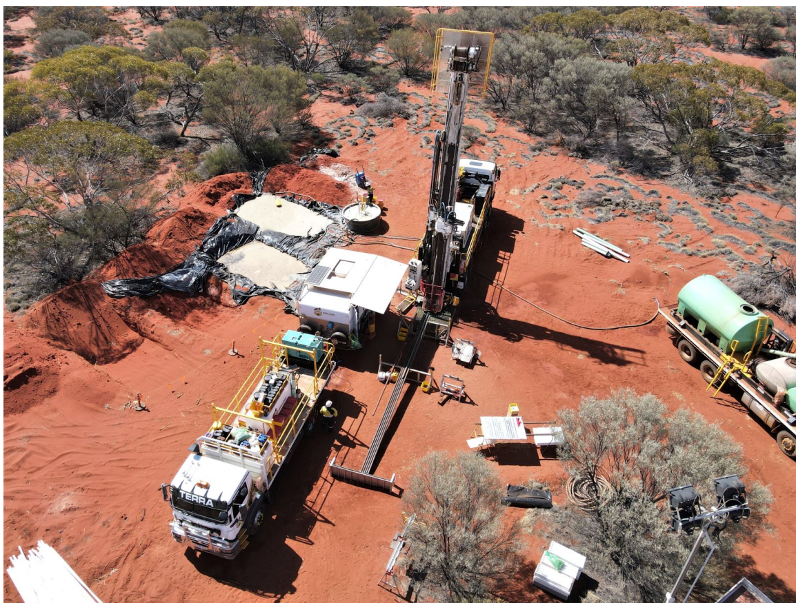
Figure 3 – diamond drilling underway at Mt Alexander.
