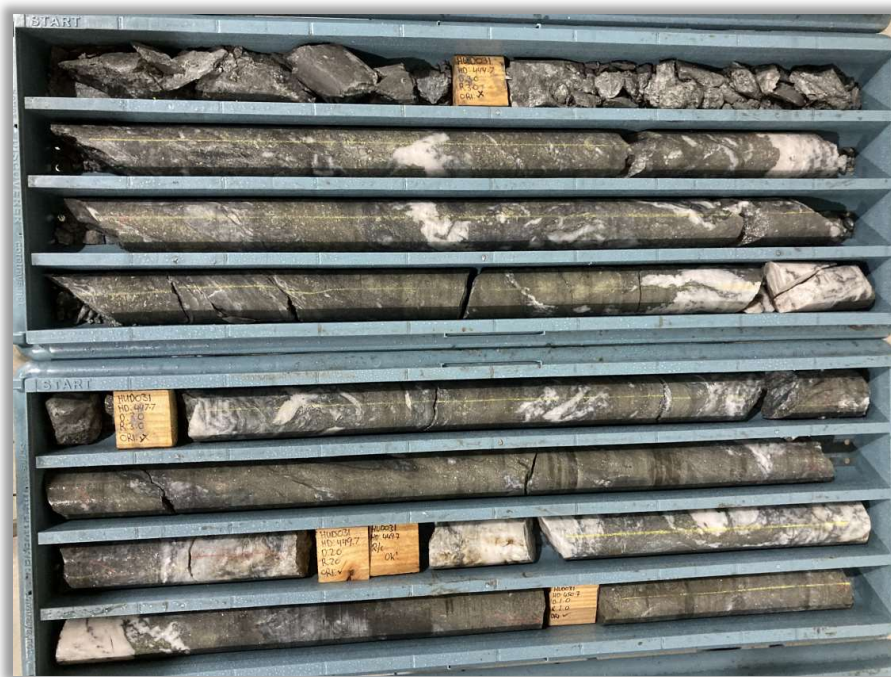
Figure 4 - Hume Target - Massive sulphides and quartz in HUD031 from 444.5m-451.0m within broader sulphide-rich interval from approximately 396m-451m - Assay Pending.
