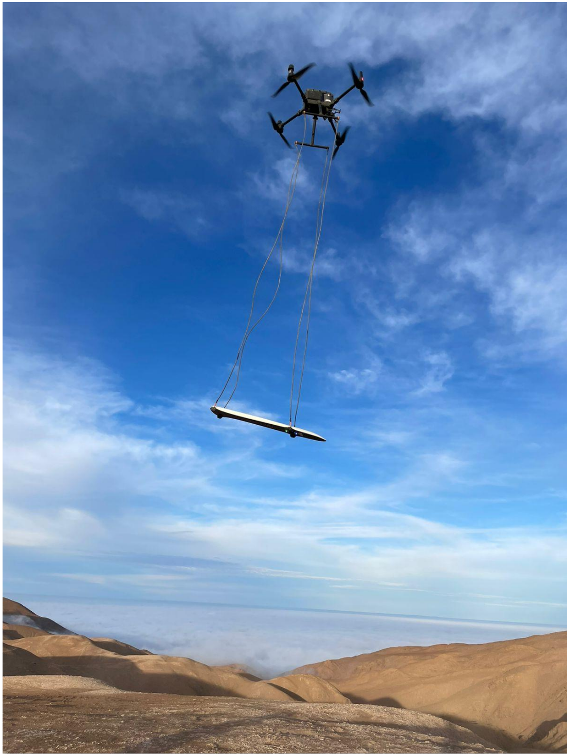
Figure 3: Drone magnetometry survey underway at Ilo Norte
