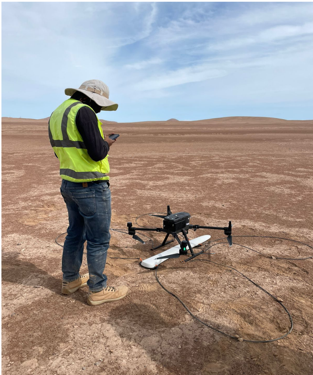
Figure 4: Real Eagle contractor with drone mounted magnetometer operating at Ilo Este
