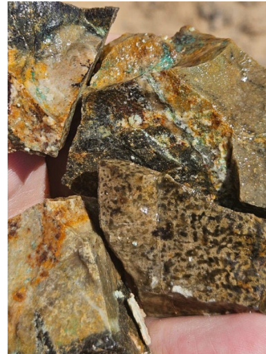
Figure 8: Hornfels, some with secondary biotite, with green and black copper oxides in fractures associated with quartz. Multiple generations of fine quartz veining indicate more than two hydrothermal events (262100E, 8060641N)
