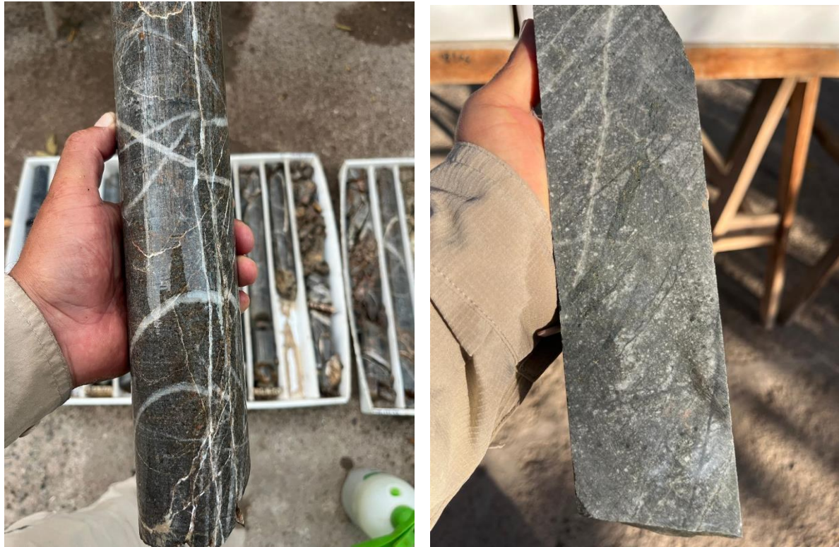
Figure 1 (left image): IE-001-2025 drill core from 177 to 180 metres showing potassic alteration and stockwork. Visually estimated grade 0.1 - 0.4% Cu. Laboratory assay results are due to be received in September 2025.
