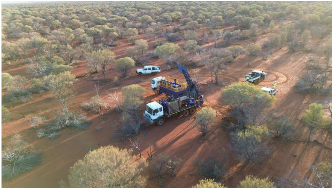
Figure 5: Aircore drilling in soil-covered terrain at Bunjarra.
