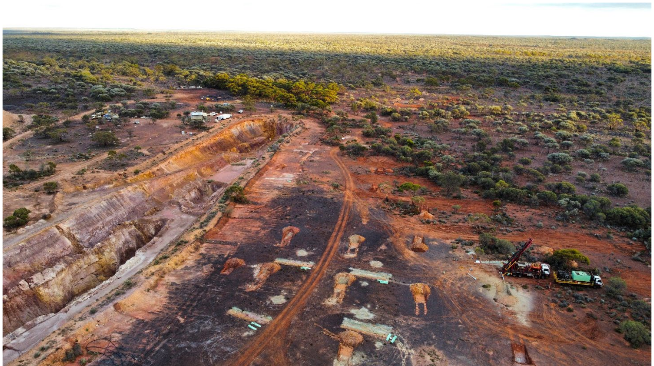
Picture 1: RC drill rig on site at Zelica targeting depth extensions of known mineralisation below pre-existing shallow open pit on the left (looking NNW)
