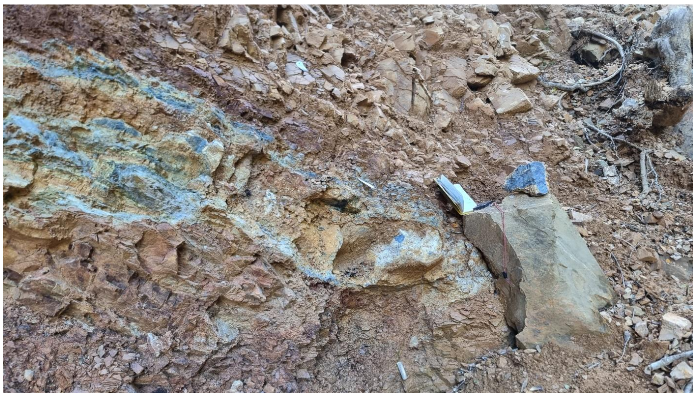
Figure 7: The Skyline Reef with 0.4m Thick Massive Stibnite Vein on the Hanging wall (location of Channel Samples No 8 and 8a).
