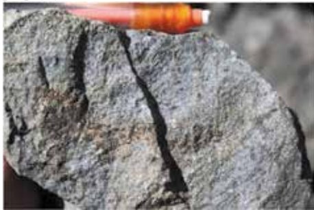
Plate 11. Chalcopyrite-quartz-actinolite bearing vein in andesite, Marietta Mine.
