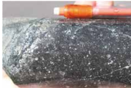
Plate 26. Feldspathic volcaniclastic breccia with strong biotite-albite alteration and disseminated pyrite \pm chalcopyrite, 408.3m YS002RCD
