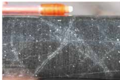
Plate 28. Quartz-magnetite-actinolite bearing A-style veins in biotite-magnetite altered volcaniclastic breccia, 414.5m YS002RCD.
