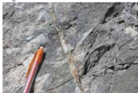
Plate 18. Quartz-epidote-chalcopyrite bearing B-style vein, Brocky Target
