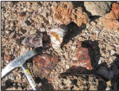
Plate 35. Sub-crops of quartz-breccia and vuggy quartz, which reported 1.93g/t Au (Figure 25)
