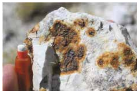
Plate 16. Strong silica calc-siltstone and strong quartz-garnet-epidote-Cu oxide veins, Brocky, Target.
