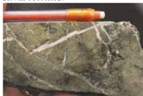
Plate 24. Strong sericite-carbonate alteration overprint on biotite-magnetite altered volcaniclastic breccia in a fault zone, 274.1m YS001RCD.
