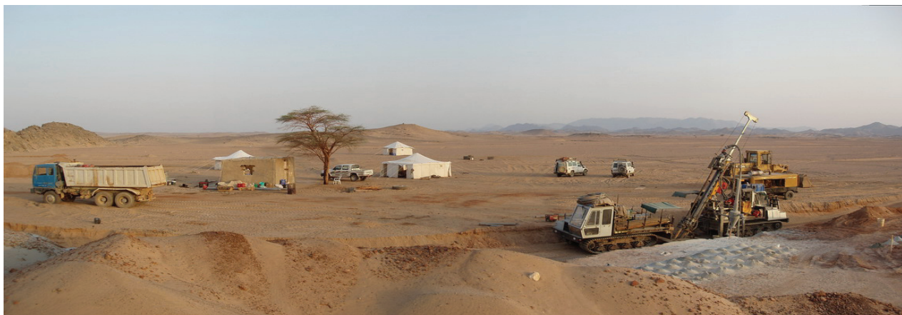
Figure 6: RC drilling operations at Abu Swayel
