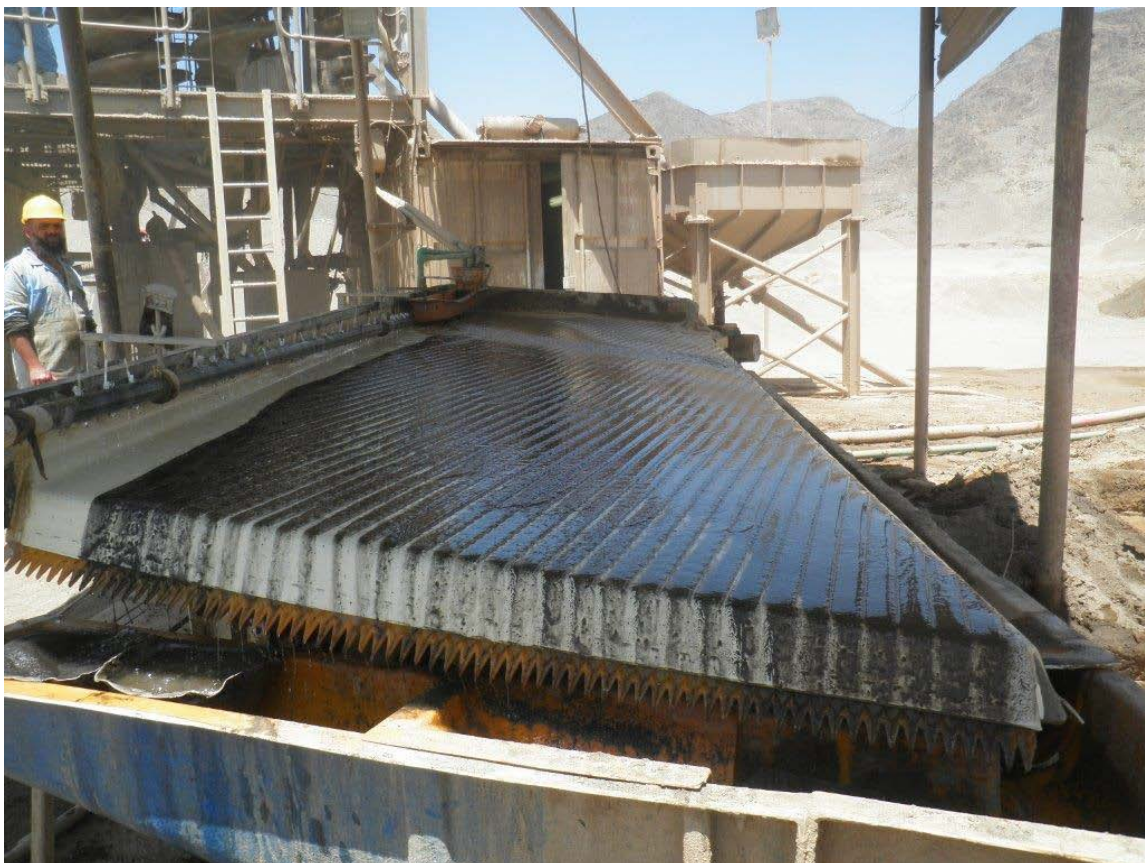
Figure 4: Wilfley Table at the Abu Dabbab Alluvial Mining Project
