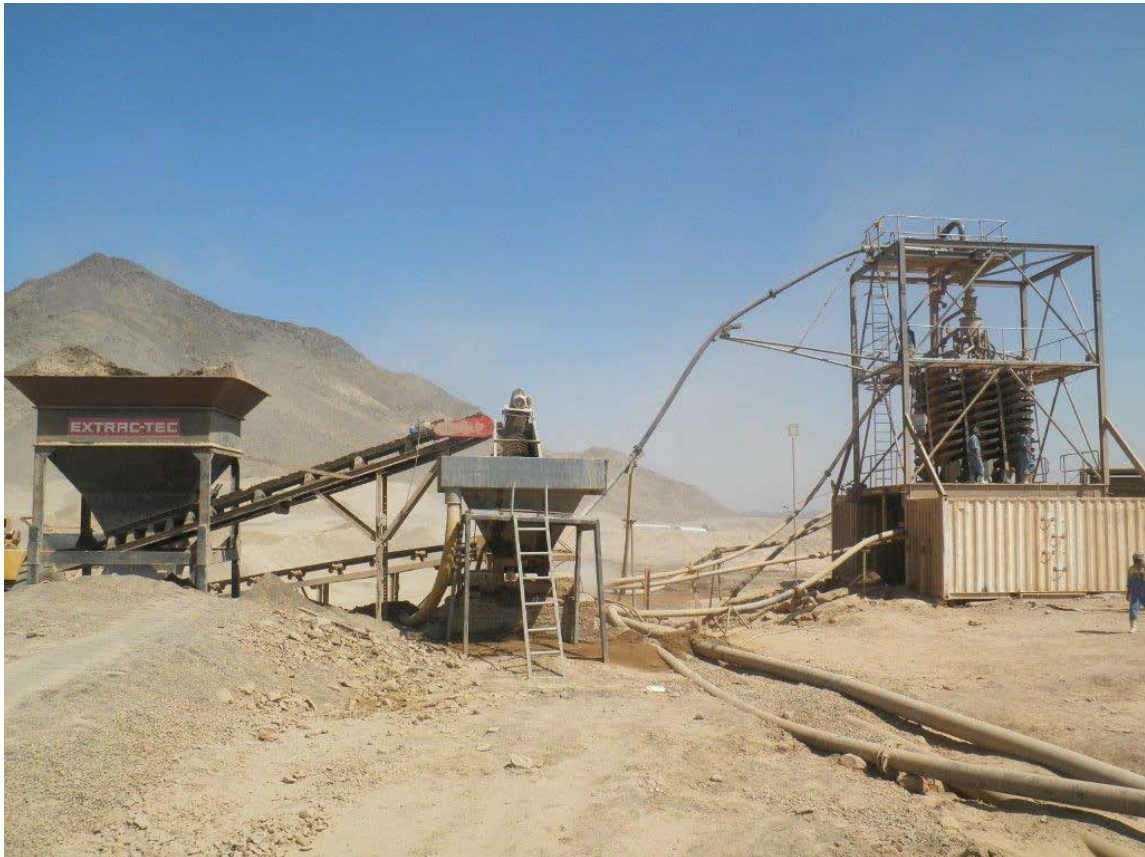
Figure 3: DMS Circuit and Spiral Plant at the Abu Dabbab Alluvial Mining Project
