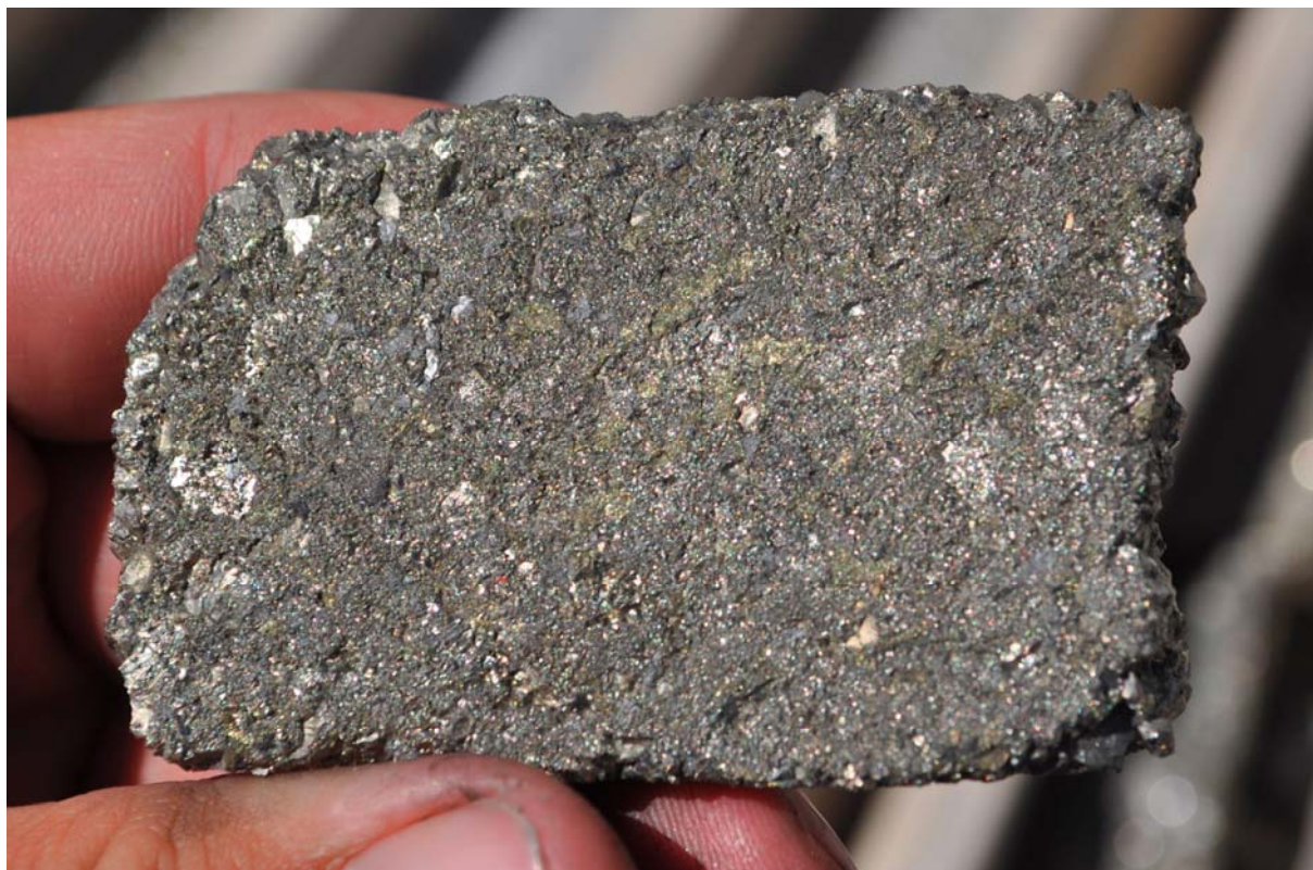
Photograph 1. Close-up photograph of halved NQ drill core from drill hole SPOM023 showing chalcopyrite ( \text{CuFeS}_2 ) (yellow) in massive pyrite ( \text{FeS}_2 ) (silver-grey).
