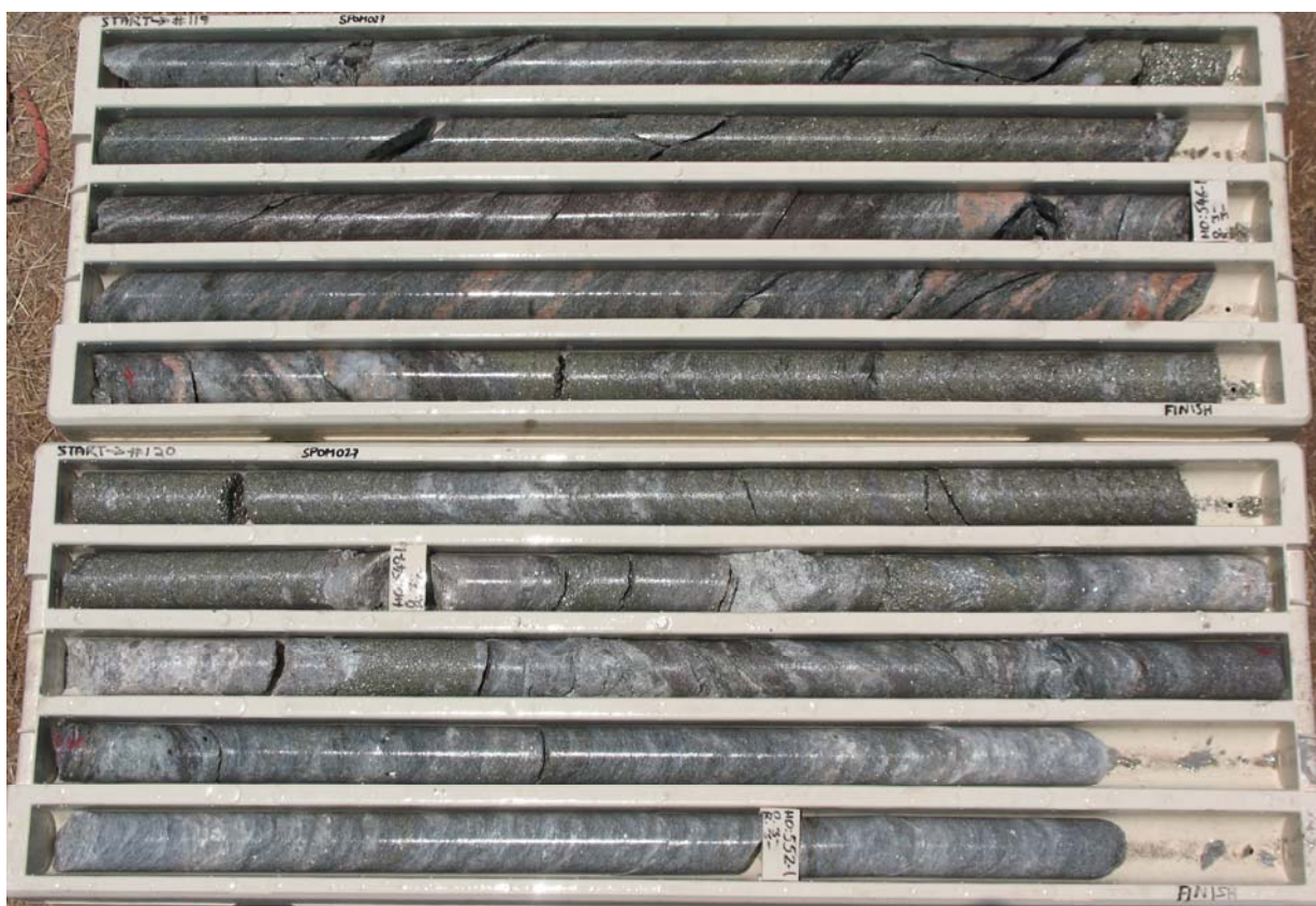
Photograph 3. Semi-massive sulphide intersections between 543.0m and 550.1m in drill hole SPOM027 at One Mile. NQ core diameter is 47.6mm and length of a tray is 1 metre.
