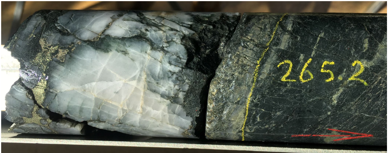
Figure 7. BTDD005 – quartz-pyrite-chalcopyrite vein at 265.2m
