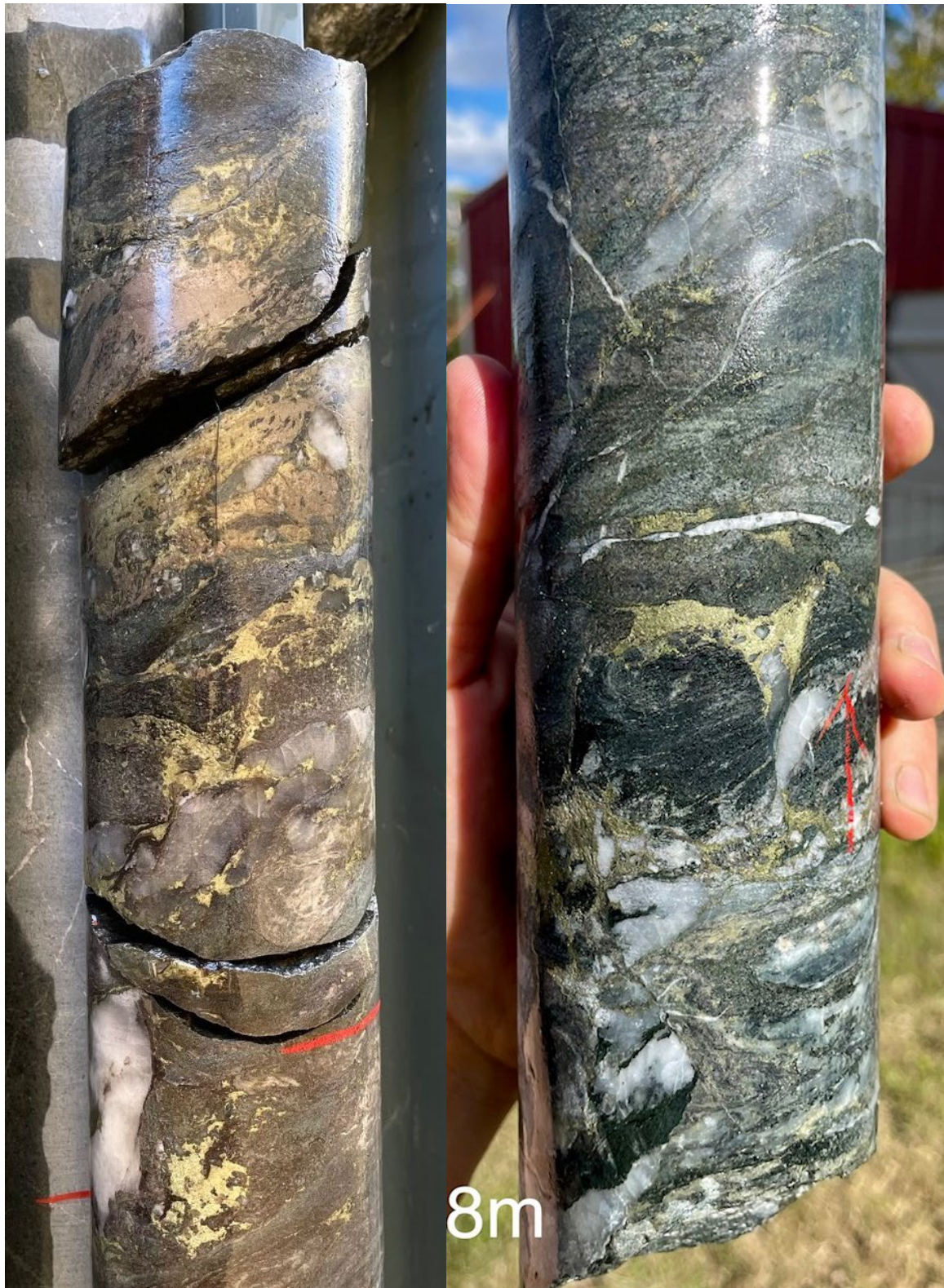
Figure 10. BTDD006 – 531.7m (left) - quartz-pyrite-chalcopryrite-pyrrhotite; 491.8m (right) – breccia infill quartz-pyrite-chalcopryrite-pyrrhotite
