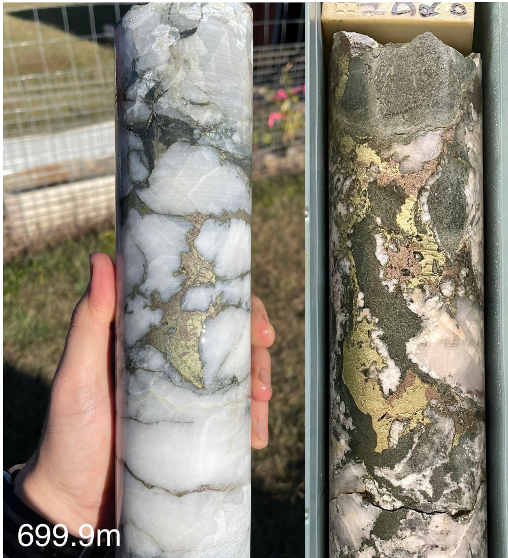
Figure 8. BTDD005 – 699.9m (left), 708.5m (right) – buck quartz vein with chalcopyrite-pyrite-pyrrhotite infill.
