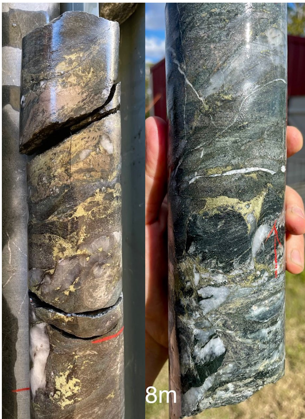
Figure 7. BTDD006 – 531.7m (left) - quartz-pyrite-chalcopyrite-pyrrhotite; 491.8m (right) – breccia infill quartz-pyrite-chalcopyrite-pyrrhotite.
