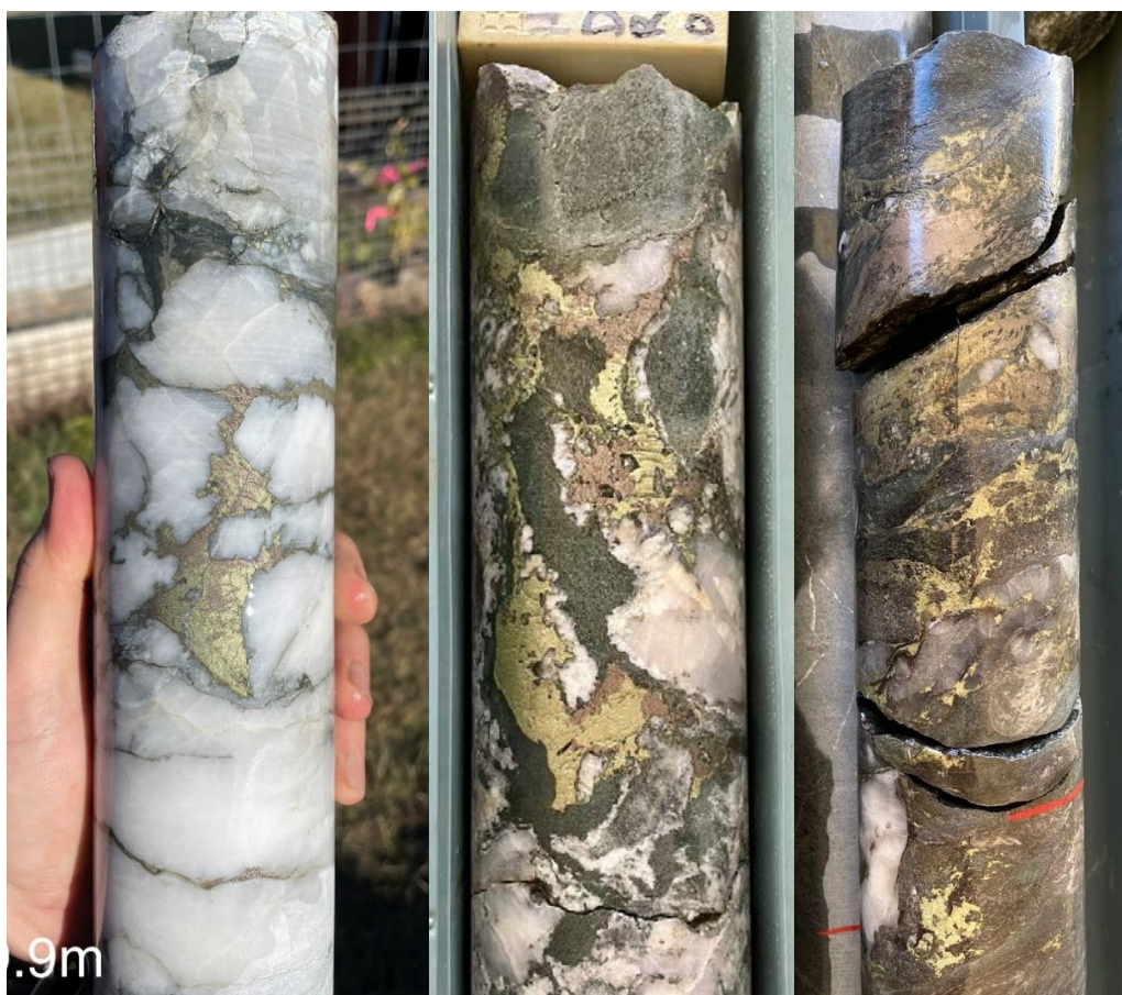
Figure 21. Examples of wall rock-hosted vein mineralisation: BTDD005 – 699.9m (left); BTDD005 – 708.5m (middle) – buck quartz vein with chalcopyrite-pyrite-pyrrhotite infill; and BTDD006 – 531.7m (right) – quartz-pyrite-chalcopyrite-pyrrhotite.
