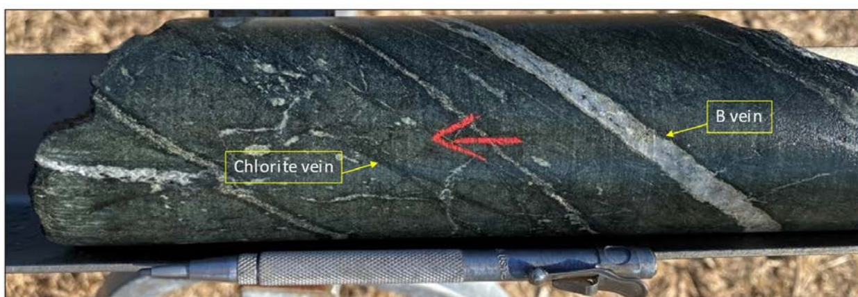
Figure 10. Core from CCDD001 (30.25m) showing meta-andesite unit with a porphyry B vein containing quartz, pyrite and chalcopyrite. Fine chlorite veining with patches of epidote alteration also present.
