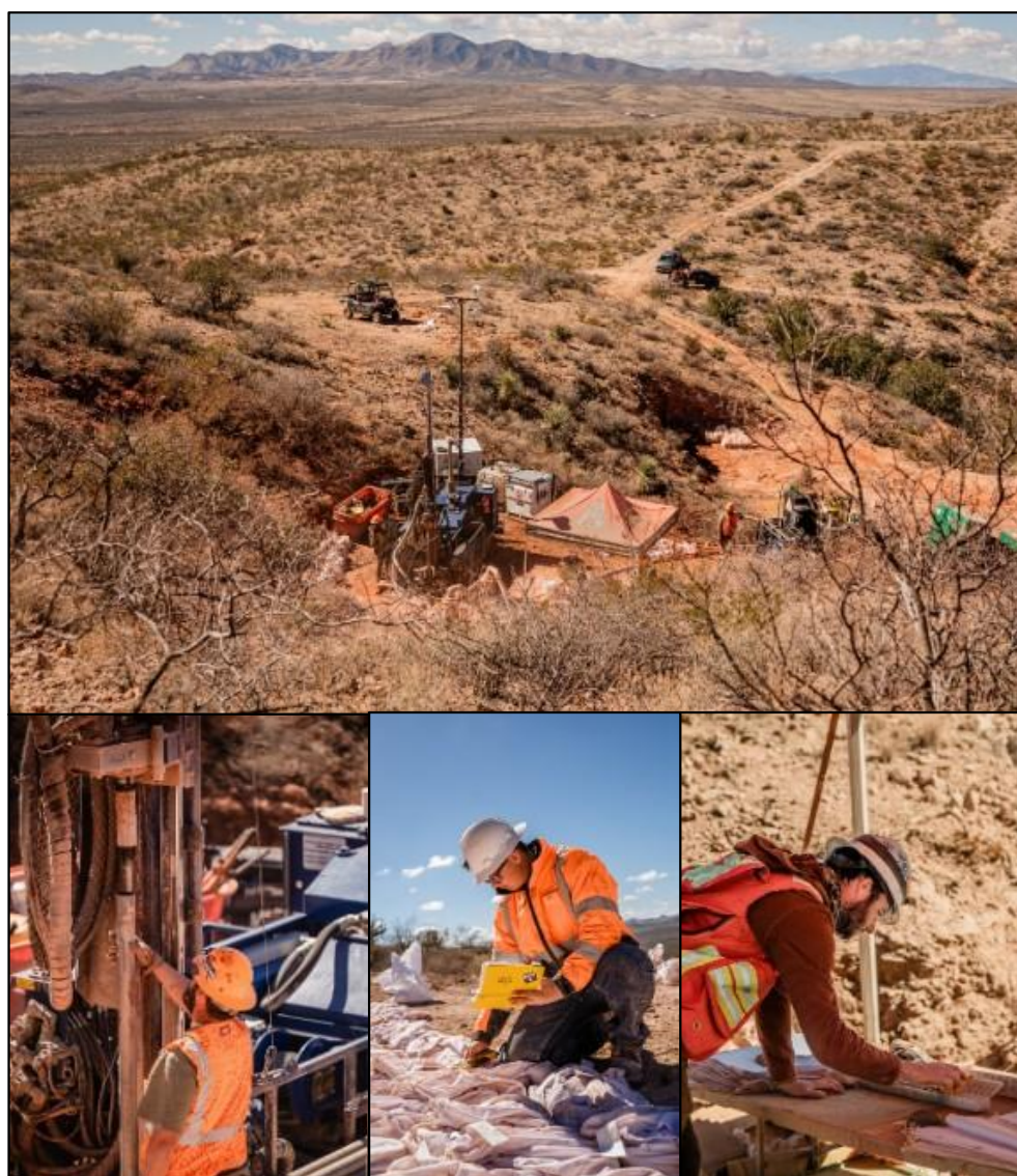
Figure 1: Clockwise from top. Midnight Sun's Grasshopper RC rig drilling RBRC026. Company geologist inspecting RC chips. Field technician collecting magnetic susceptibility measurements. RC drilling rod change.
