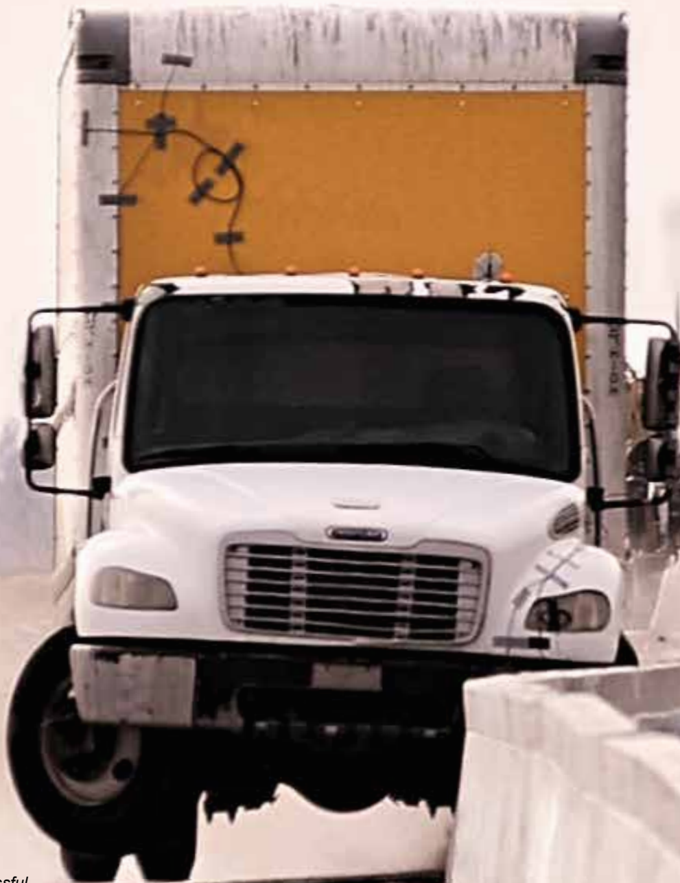
HV2™ Barrier successful TL-4 crash test - January 2018
