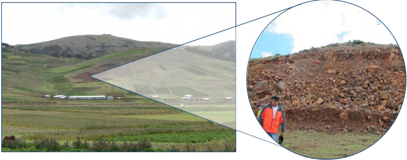
Figure 16: Opaban I deposit has favourable topography for low strip-ratio, open cut mining
