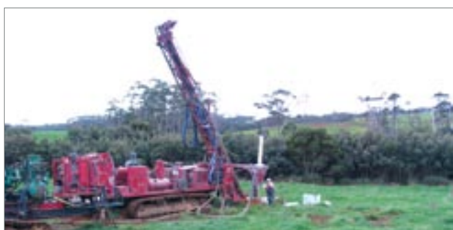
Stellar RC drilling at Gourlays Creek
