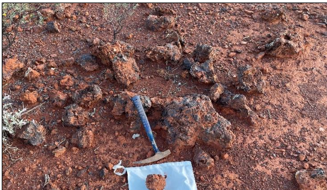
Figure 4: Outcropping gossan at Baxters returning pXRF values of 0.11% Cu, 0.1% Zn, 130ppm Pb and 0.11% Ba.
