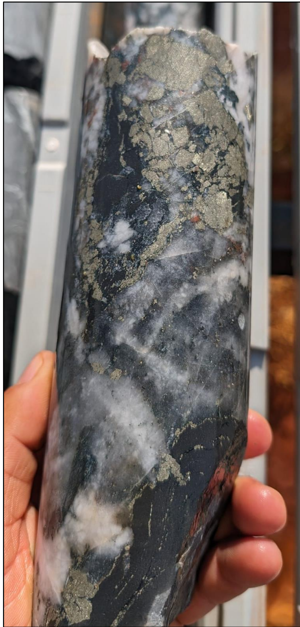
Figure 4: MRDD004 drill core (260.45 to 260.7m), showing intense quartz carbonate veining (50% quartz carbonate veining) with approximately 20% pyrite content.
