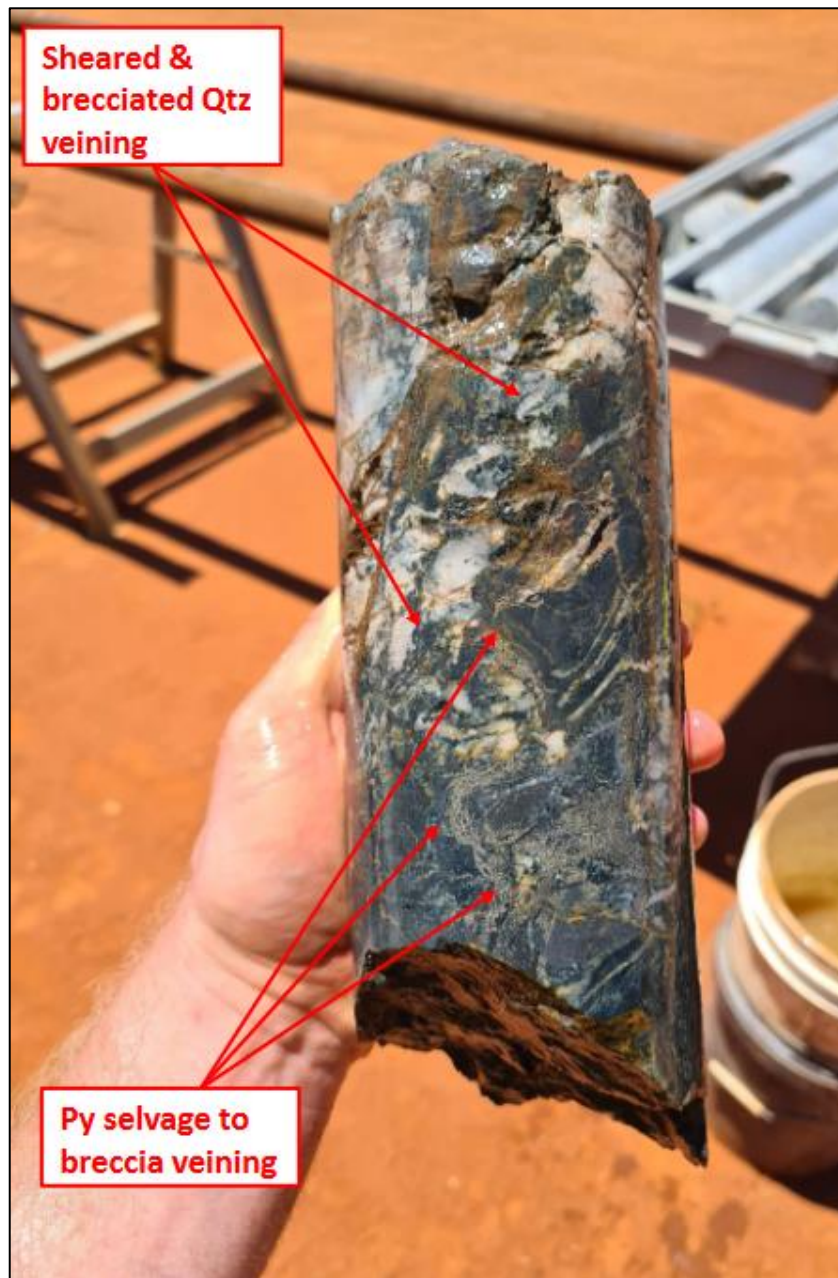
Figure 2: MWDD001 drill core (125.3m to 125.5m) - brecciated SIF unit with approximately 4% sulphide content proximal to 15% quartz carbonate veining
