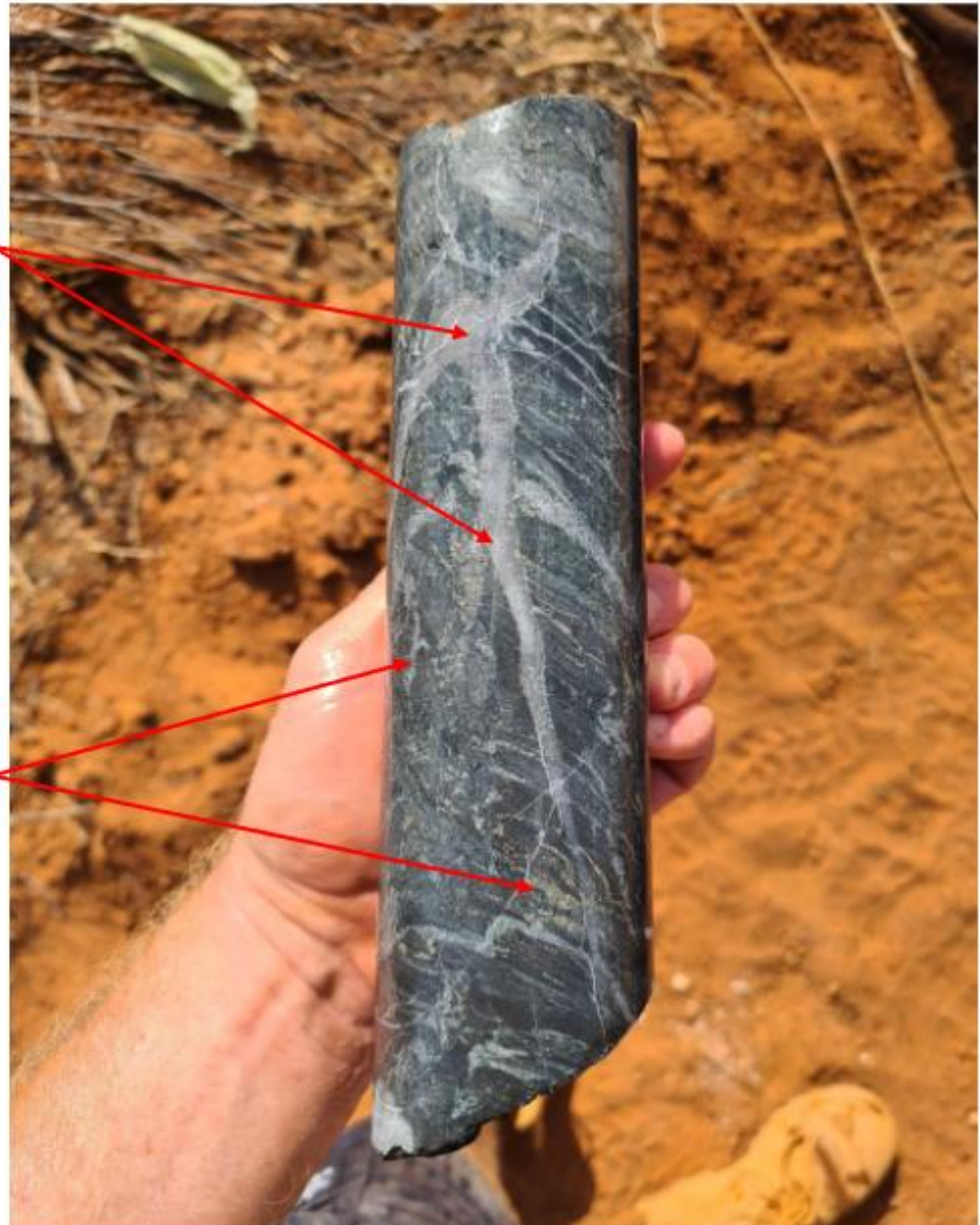
Figure 3: MWDD003 drill core (208.2 to 208.5m) – intense quartz carbonate veining (approximately 10%) with 3% pyrite content
