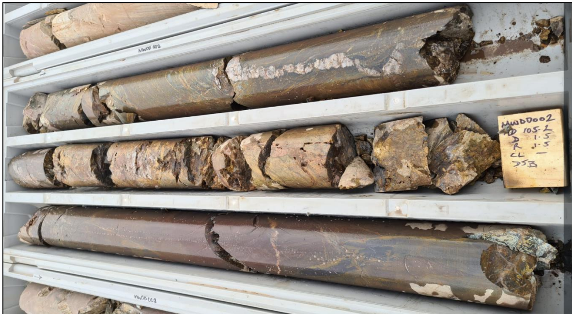
Figure 5: MWDD002 drill core (103.5 to 106.3m) showing a zone of dense (estimated 20%) boudinaged, vuggy, quartz carbonate veining with 5% ex sulphide content within the BIF saprock. This intersection is a 40m projection south from discovery hole HWAC1472.
