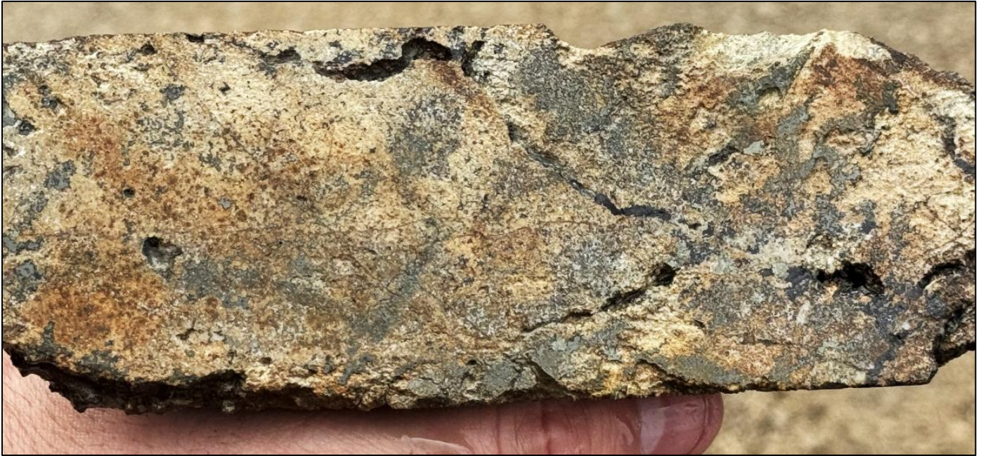
Figure 5: Core photo of replacement-type, silica altered green garnet skarn with semi-massive sphalerite-galena in ZRSD25213 from 400.0m to 402.1m – 6.5g/t AuEq 2 (2.2g/t Au, 2.8% Pb, 5.4% Zn & 20.4g/t Ag).
