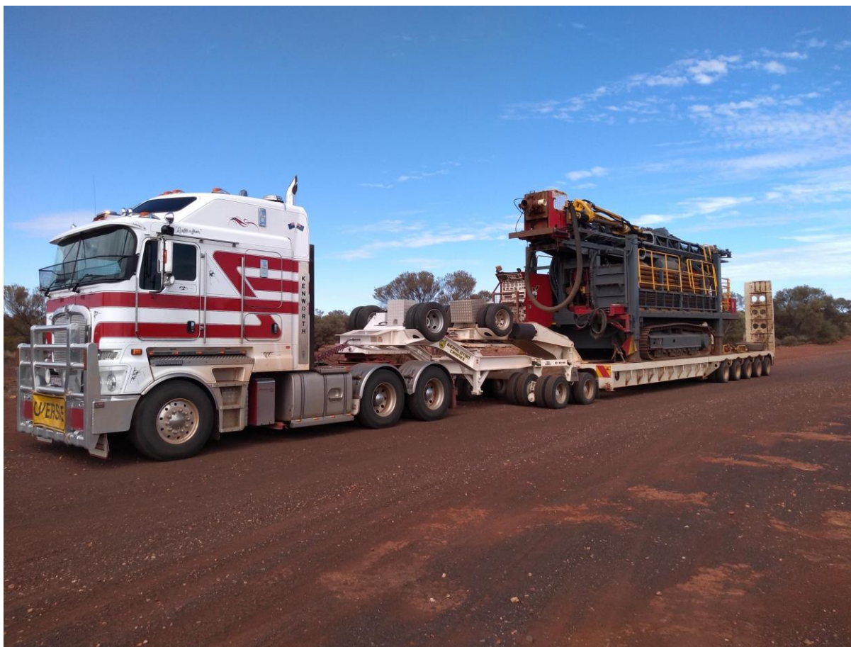
Figure 2 Track mounted RC drilling rig arriving at Apollo Hill – 23 March 2019. A track mounted drill rig is being used to improve access to several drill pads on the lakeshore at Apollo Hill and to several drill pads on the side of Apollo Hill; drill pads being used respectively to test Apollo Hill southern extensions and hanging wall lodes.
