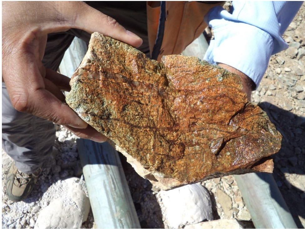
Figure 7.2_3 Hand Specimen – Typical Veining within Central Porphyry Zone
