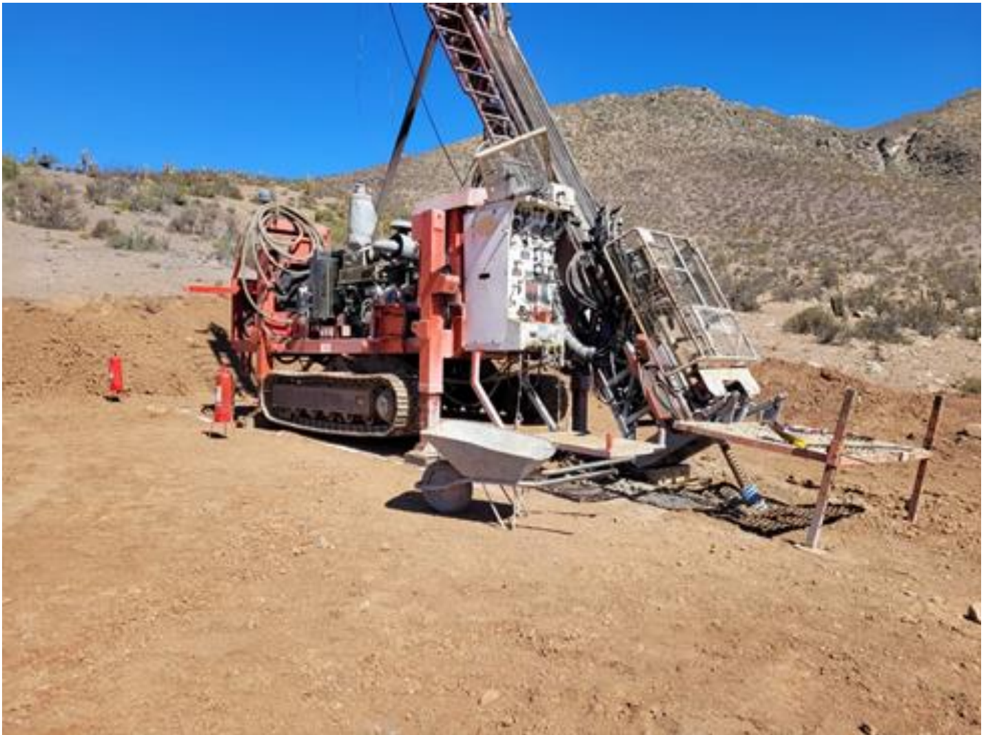
Diamond drill rig in operation at Colina2
