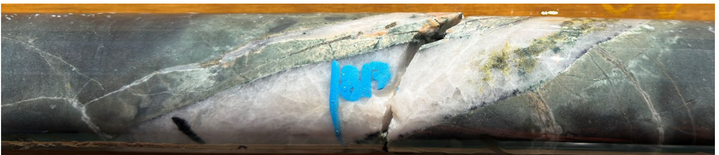
Photo 1. Molybdenite mineralisation in quartz vein 817 m downhole in 26LHDD073* (refer to Appendix 1).
