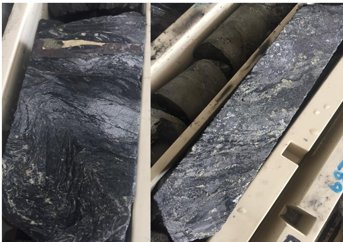
Photo 2. Massive sulphide mineralisation at Bowdens Silver showing high concentrations of sphalerite, galena and pyrite.
