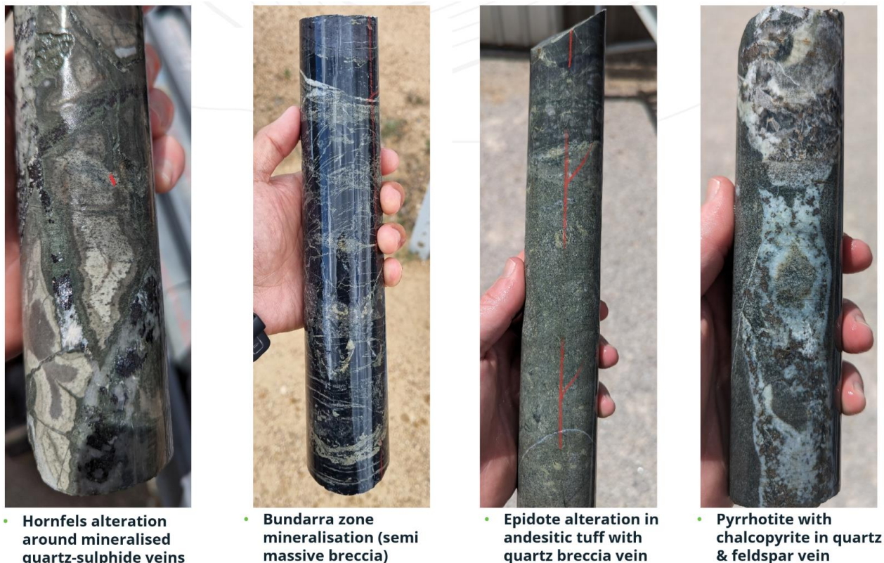
Figure 5: Selection of drill core from the three deep drill holes displaying alteration and mineralisation at depth.
