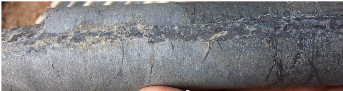
Figure 7.3.7 NQ Core with Steep Polyphase Vein
