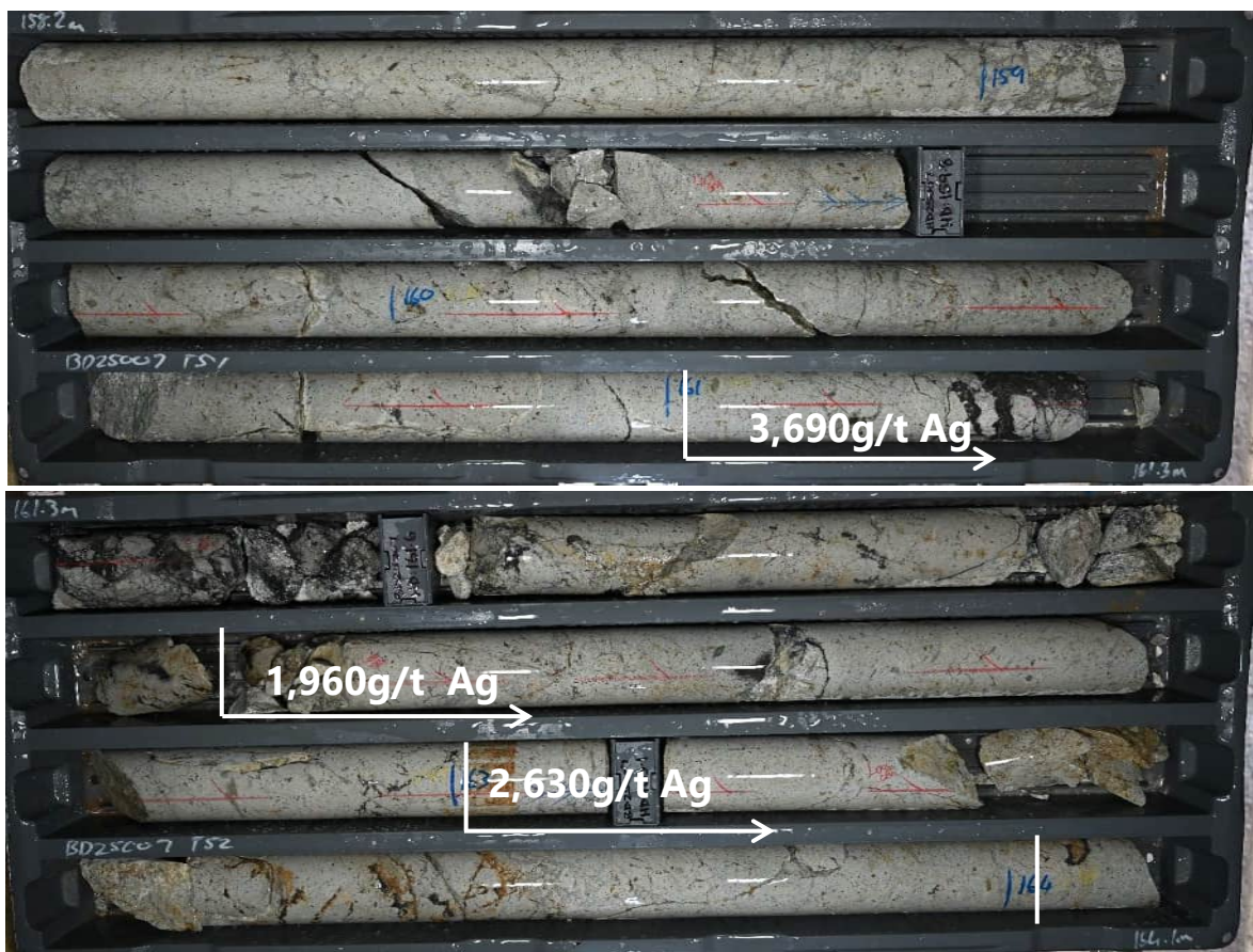
Figure 7.3.8 Fracture Fill Vein and Stockwork
