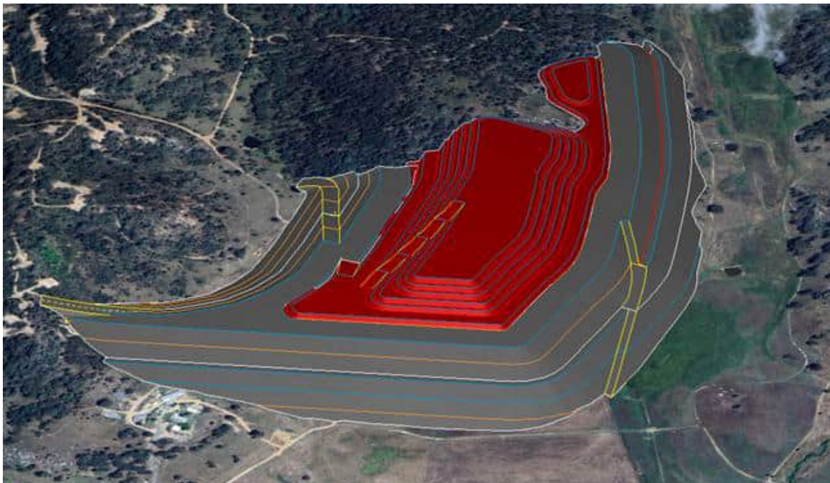
Figure 15.4.1 Main Dump, Type 1 Outer Layer and Type 3 PAF Inner Dump
