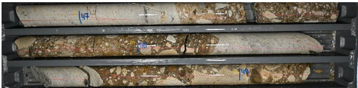
Figure 7.3.9 Hydrothermal Breccia BD25004 47 – 48 m
